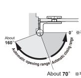
¾3 The maximum lifting of the door is 5 mm when the opening angle is 70 °.
